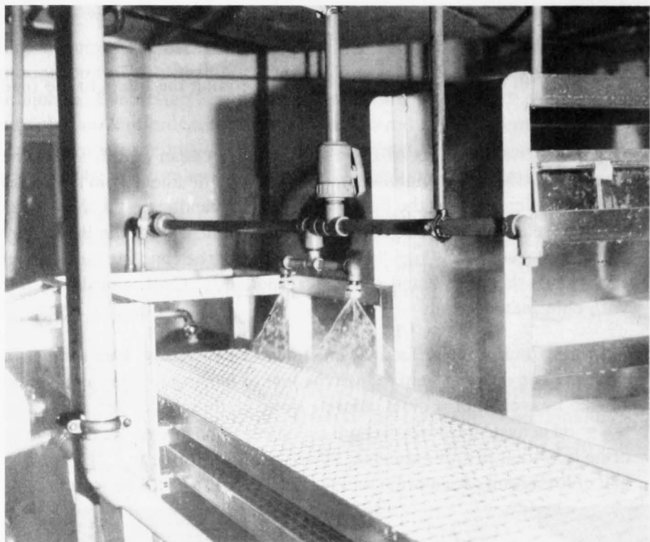
Figure 13.—Spray nozzles set at the end of a stainless steel fillet conveyor.
