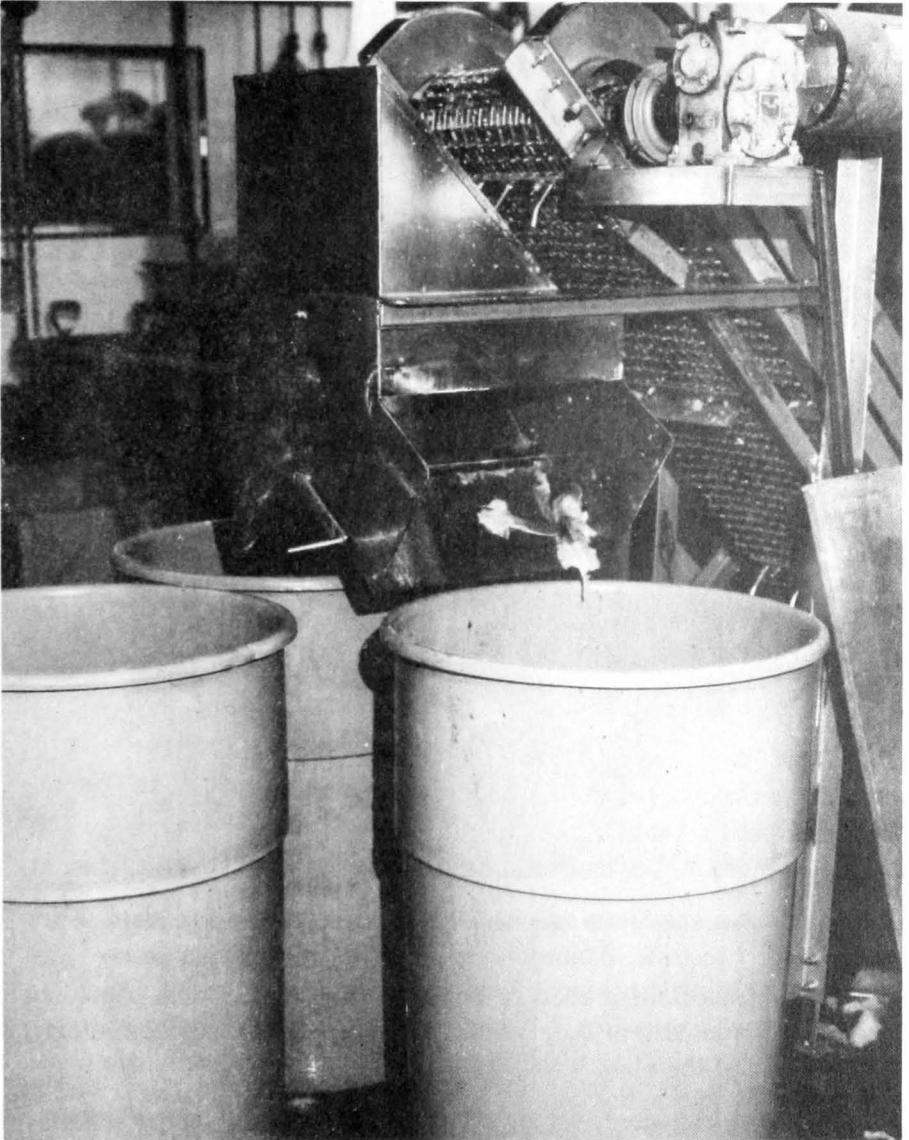
Figure 5.—Fish waste from the filleting line is conveyed directly to plastic containers which are used only for this purpose.
